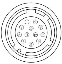
Fig. 2. 12 pin connector
